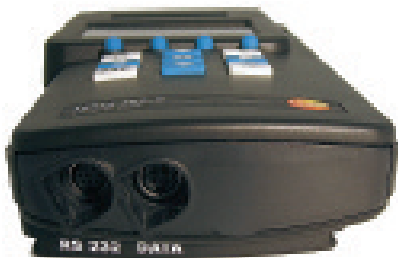
RS 232 connection Remote cable connection
